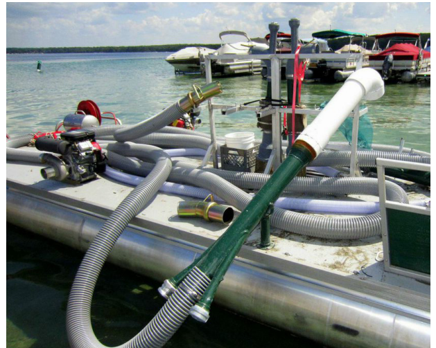
Figure 10. Diver-assisted suction harvesting.
